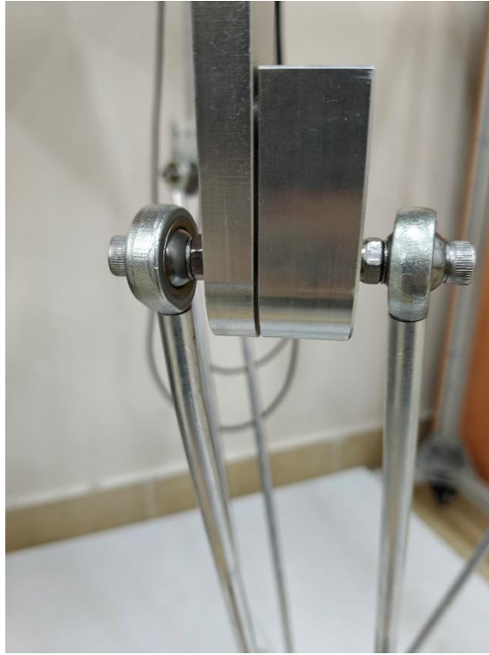
Figure 6.15. Original Joint with M10 Bolts Photograph showing original oversized hardware configuration.
